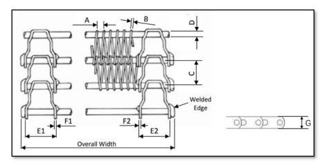
**NOTE:** When measuring pitches A & C, it is best practice to measure over 10 pitches and divide by 10 to obtain the average pitch.
